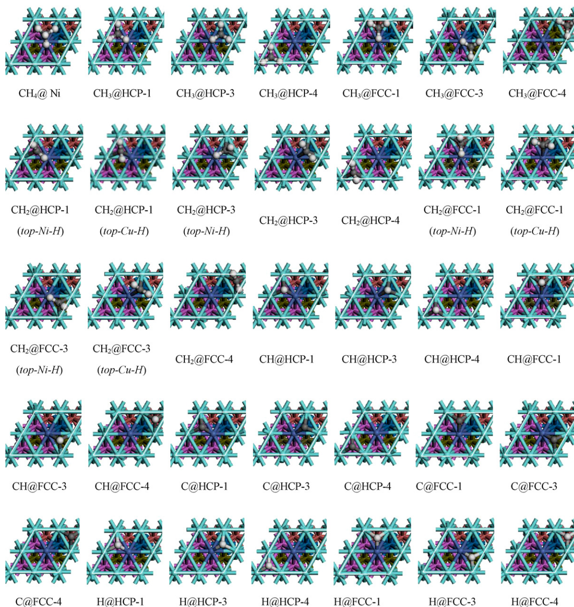
Fig. 3. The adsorption configurations of the \text{CH}_x ( x=0-4 ) on Model B of NiCu (111).
